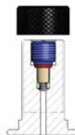
Model of valve stem integrated 5/8" 18 UNF (D)
