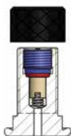
Model of valve stem integrated 7/8"14 UNF (C)
