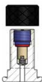
Model of valve stem integrated 7/8"14 UNF (C)
