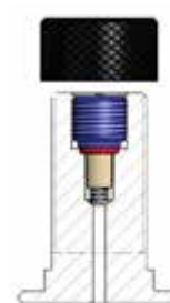
Model of valve stem integrated 5/8" 18 UNF (D)
