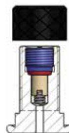
Model of valve stem integrated 7/8" 14 UNF (C)
